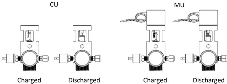
3. Remove and weigh the complete unit (without brackets) on a certified scale every six (6) months and record on tag provided.
