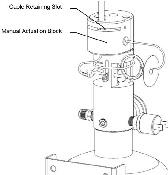
Insert extinguisher end of Cable through hole in Manual
