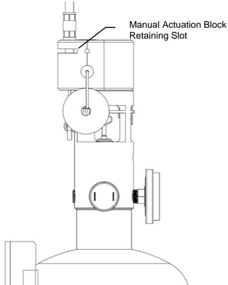
Align retaining slot of Cable with retaining slot of Manual
