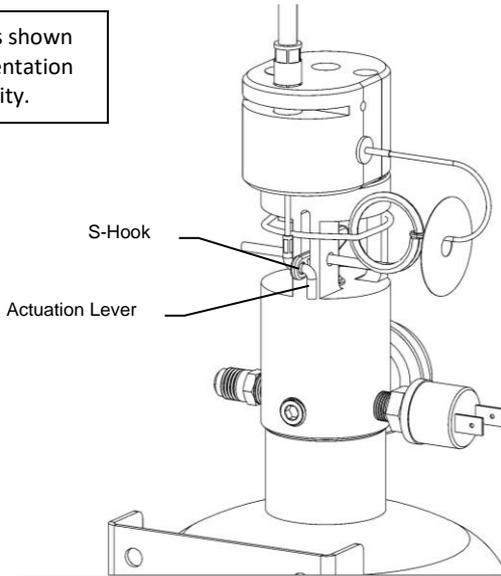
Insert S-Hook into hole of Actuation Lever.
